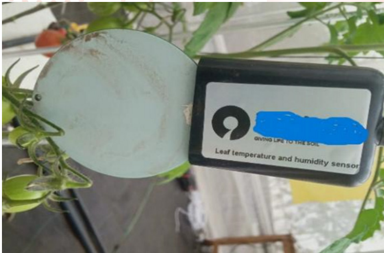
Leaf wetness sensor installed to forecast fungal disease development stages on greenhouse tomatoes for decision making; whether to initiate treatment or prevention actions.
