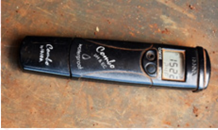
Electrical conductivity meter to determine PH and EC of coco peat
