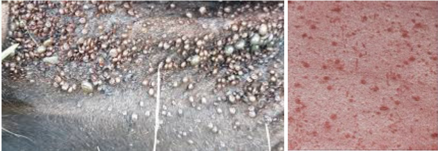
Ticks on hides (LEFT) cause pinpoint holes and blisters that persist on processed leather (RIGHT)
